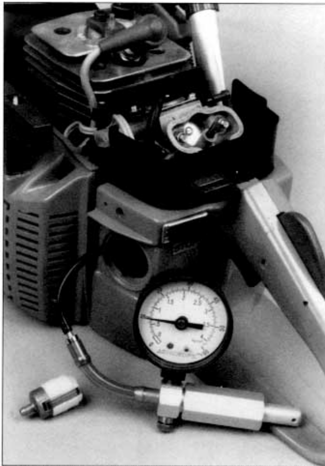
When pressure testing the fuel system, you need not wait for the inlet needle to pop off. You can open the inlet needle by cranking the engine or by tickling the metering diaphragm through the atmospheric vent hole. If the inlet needle re-seats below 10 psi, or does not re-seat, follow the procedures on p. 17 & 18.
