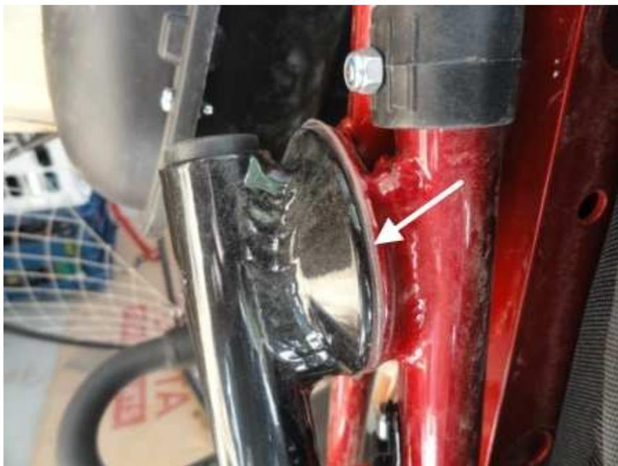
If this strap is too tight or too loose, it will strain the contact point between the bar and the frame. While sitting in the suspended harness, loosen or tighten the main chest strap so that the circular contact points on the bars are flush with the circular contact points on the frame. This adjustment will also affect the spacing between the hang points which will, in turn, affect the safe handling of the glider.
