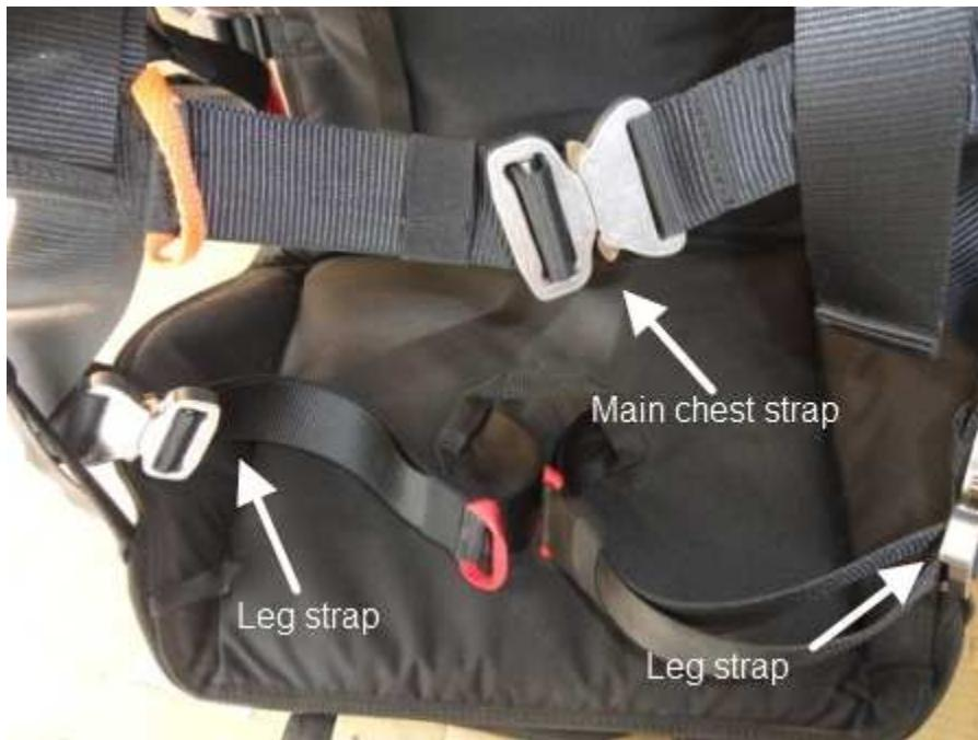
**FINAL CHECK** Sit in the harness and check all adjustments. Some of these adjustments, such as the seat angle, can be made while flying when safely away from the ground. Comfort is the most important consideration when adjusting the harness. An uncomfortable harness is a distraction and is a safety issue as a result.
