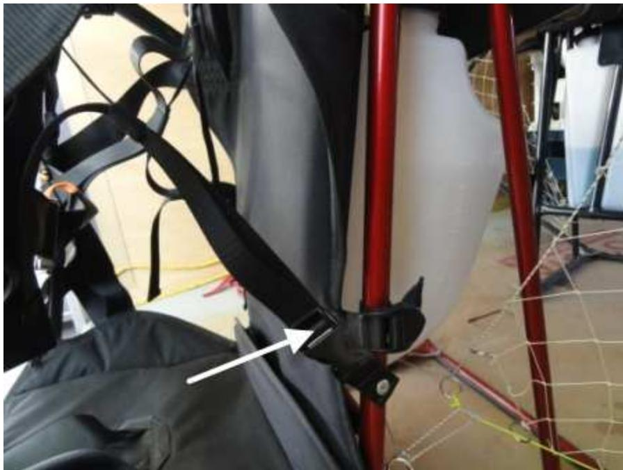
**7. CHEST STRAPS** There are two chest straps. The main chest strap (the lower of the two) must be tightened just enough to keep the suspension bars from separating around the circular contact point with the frame. In other words, there should be no space around the circular plastic disk indicated by the arrow in the photo below. This strap is primarily a safety strap.
